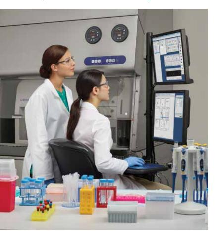
The BD FACSAria Fusion uses BD FACSDiva software to efficiently control the setup, acquisition, and analysis of flow cytometry data from the operator workstation. Software control of key operations minimizes direct interaction with the sorter for an added level of biosafety protection.
