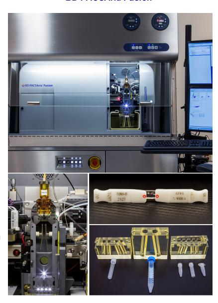
The BD FACSAria Fusion is a 20-paramater high-speed cell sorter capable of detecting 18 colors plus forward and side-scatter. Its gel-coupled cuvette allows for very accurate and sensitive measurements of fluorescence, comparable to our LSR Fortessa.
