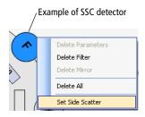
**Tip** Once SSC is set, the detector is locked. To unlock the detector, delete the parameter.
