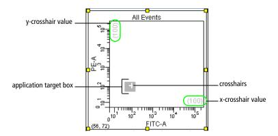
• The size of the application target box represents the SD of electronic noise of the dim beads in each detector. The default value is 2 SD, but can be set from 1 to 4 SD depending on the application. See Creating Application Settings on page 98.
