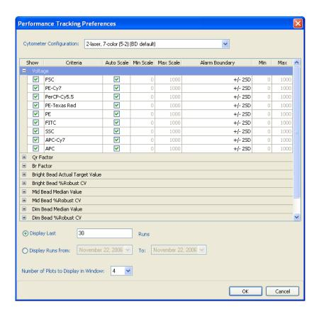
You can choose up to 20 different criteria to display under the Performance Tracking tab. Each plot displays data points for one criterion. You can display data for more than one bead lot on each plot, as shown in Figure 3-8.
