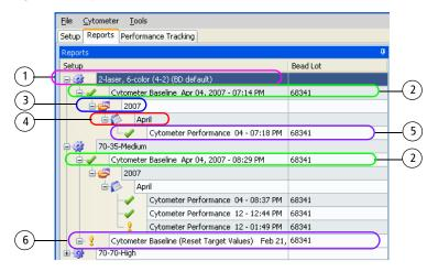
**Tip** Use the Reports view to quickly check whether a baseline has been defined, or a performance check was completed, for a specific configuration.
