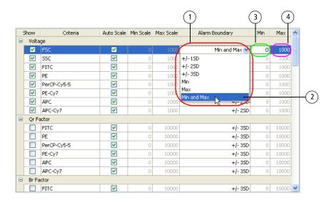
**NOTICE** Any changes made to the alarm boundaries after you have been tracking performance will not be reflected on the Levey-Jennings charts until you next run Cytometer Setup and Tracking beads.
