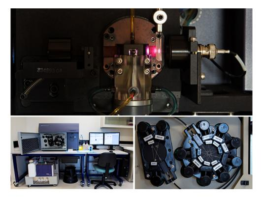
What is it? Digital flow cytometer What can it to? Flow cytometry analysis Detect 8 parameters; 6 colors 2 excitation lasers 20mW 488nm blue 17mW 633nm red -What can be run? **BSL I samples** Customization? Interchangeable filters Who can run these instruments? Technical assistance by facility staff Trained users How do I book these instruments? LDI Core Booking Calendar Where are they located? Jewish General Hospital 3999 Cote-Ste-Catherine LDI, Segal Cancer Center Room E-417
